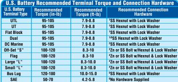
Proper connection is to position a lock washer between the nut and the connector (never between the connector and lead terminal) and apply the recommended torque or enough torque to completely compress the lock washer without deforming the lead terminal.
