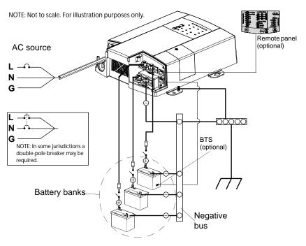
Figure 2-1 Typical Three-Battery Installation
