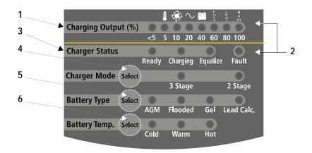
Figure 1-3 Onboard Control and Status Display Panel
