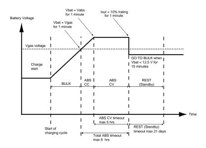
Figure 2-3 Two-Stage Charging Process
