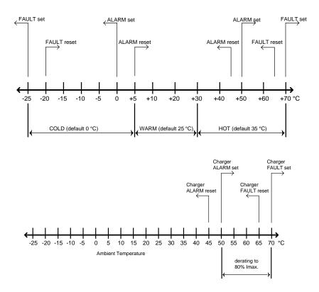
Figure 1-5 Battery and Charger Temperature Thresholds
