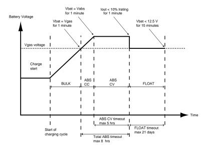
Figure 2-2 Three-Stage Charging Process
