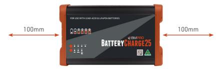
Securely mount the BatteryCharge25 to any sturdy indoor surface using the four pre-drilled mounting holes. Each mounting hole is approximately 3.7mm in diameter.
